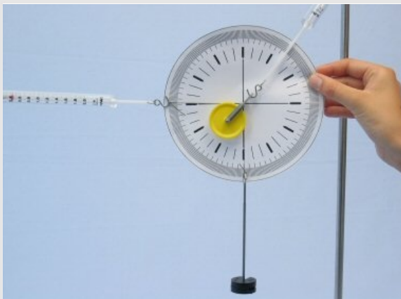
Positioning of the angle scale in the experimental setup for angles \alpha = 90^\circ
